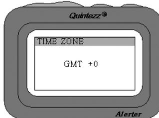
GPS satellites use the English wintertime and will be shown in the ALERTER. You can enter the time difference for your location here. Press the 'VOL-' and 'VOL+' button to change this setting to the time difference from your location to the GMT time.
