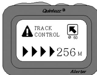
This alert indicates the start of a track control warning at a distance of 256 meter with a speed limit of 50 km/h on the current road. Please check your speed and slow down in case. At a distance of 500 meter of the camera you will hear 'TRACK CONTROL' and at a distance of 300 meter the ALERTER will say 'BE CAREFUL'.
