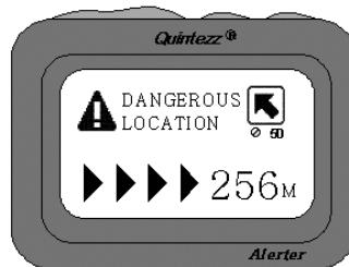
This alert indicates a dangerous location at a distance of 256 meter with a speed limit of 50 km/h on the current road. Please check your speed and slow down. At a distance of 500 meter of the location you will hear 'DANGEROUS LOCATION' and at a distance of 300 meter the ALERTER will say 'BE CAREFUL'.
