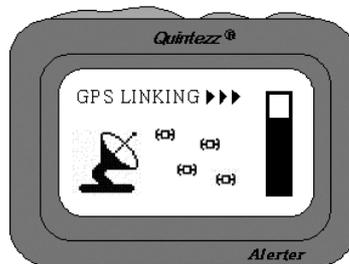
As soon as a connection has been established with at least 4 satellites, the ALERTER is showing 'GMT date'. This date and time is the 'Greenwich Mean Time', which is independent from summer- or wintertime. Now it is able to execute a reliable positioning, and all functions of the ALERTER will be available.
