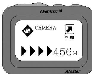
While driving, the ALERTER will give a warning sound when you approach a camera, a dangerous location, a track control section or a user data location. This audible warning depends on your setting for the 'Clock Bell'. In case this setting is OFF, there will only be a warning in case of overspeed.
