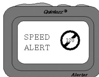
There are two kinds of speed alert warnings showing the above display: 'warning limit speed alert' and 'system limit speed alert'. In case of a 'warning limit speed alert', you will hear a 'DING DING DING' tone. In case of a 'system limit speed alert', you will hear 'TING TING TING' with a sharp tone.
