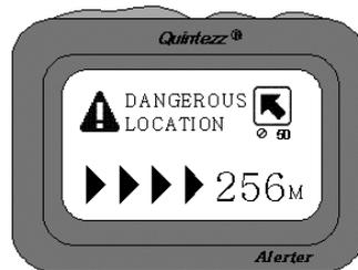
This alert indicates a dangerous location at a distance of 256 meter with a speed limit of 50 km/h on the current road. Please check your speed and slow down. At a distance of 500 meter of the location you will hear 'DANGEROUS LOCATION' and at a distance of 300 meter the ALERTER will say 'BE CAREFUL'.
