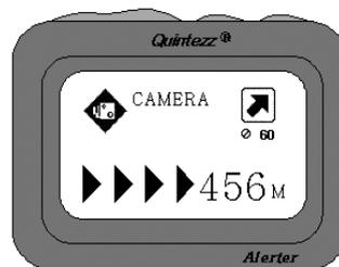
While driving, the ALERTER will give a warning sound when you approach a camera, a dangerous location, a track control section or a user data location. This audible warning depends on your setting for the 'Clock Bell'. In case this setting is OFF, there will only be a warning in case of overspeed.
