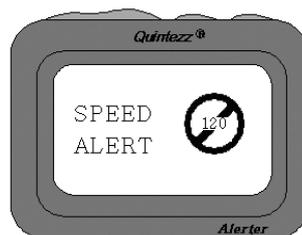
The user can switch off this feature by selecting 'SPEED ALERT OFF', which is 0 KMH!
