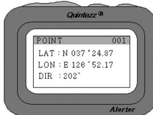
The user can manually add and delete locations from the ALERTER memory while driving. These locations are called 'user data' and can be exchanged with other people using the ALERTER. In this submenu, it is only possible to view the user data locations. It is not possible to add/change/delete locations in this submenu.
